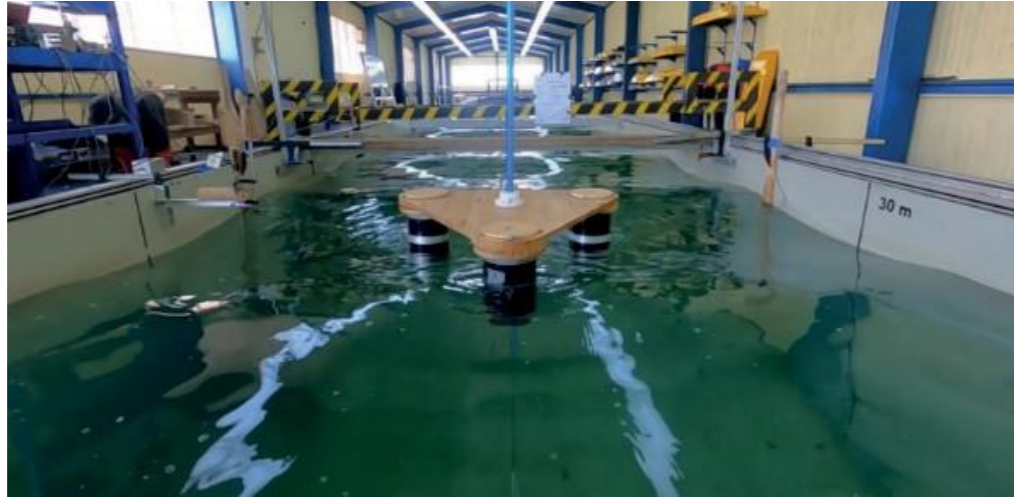
Fig. 10: Model-scale tests of generic floating wind platform at CEH-UACH.
